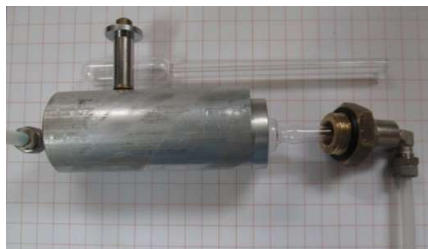
Figure 4 – Vial holder used to introduce the radon contained in glass vials into the radon reference measurement system. The small vertical cylinder on the top of the vial holder is used to break the vial and transfer the radon into the circuit.
