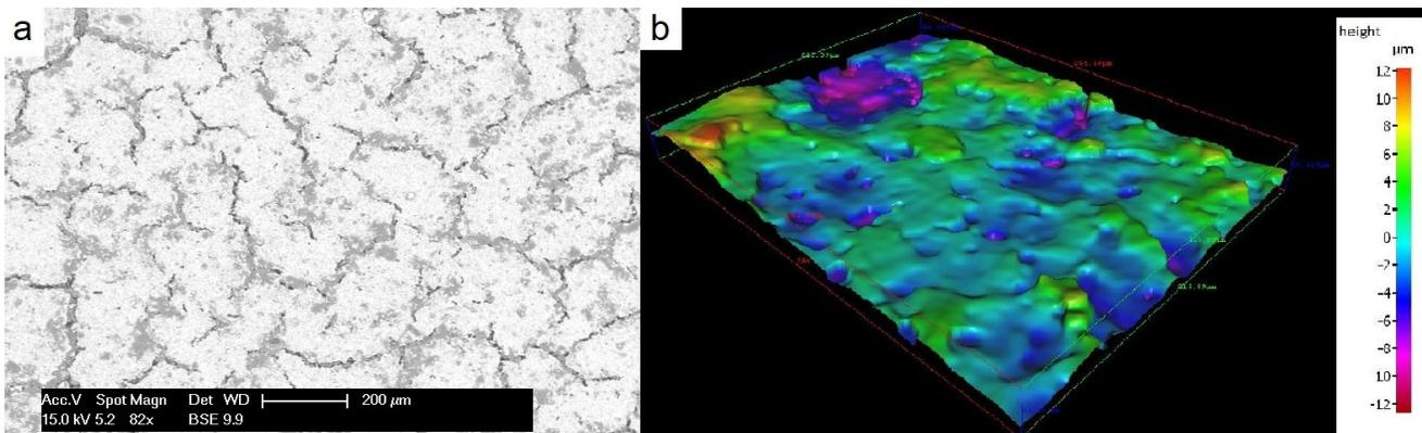
**Figure 6.** (a) SEM image of the surface of protective layer coated on 304L stainless steel substrate, crosslinked at 200 °C and pyrolyzed at 700 °C in argon; (b) 3D topography measurement of the layer.
