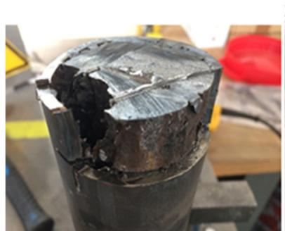
**Figure 9.** Small representative component coated with protective layer after test in AlSi<sub>12</sub>.
