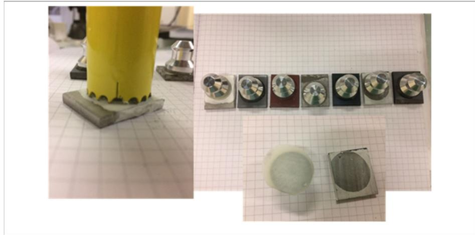
**Figure A2.** Automatic adhesion tests.
