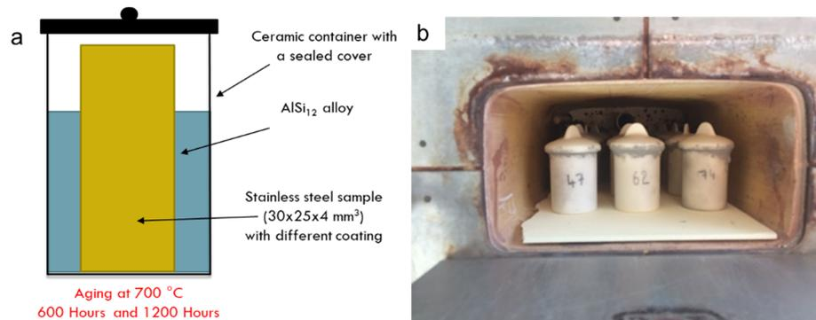
**Figure 1.** Corrosion resistance of a 304L stainless steel coated with a protective layer in molten AlSi<sub>12</sub> during 600 and 1200 h at 700 °C (a) schematic view and (b) ceramic containers in the furnace.
