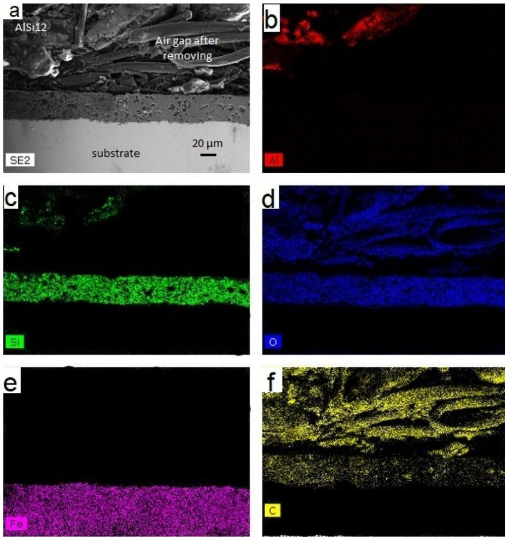
**Figure 8.** (a) Cross-sectional SEM observation of the protective layer coated on the 304L substrate after 1200 h at 700 °C in AlSi<sub>12</sub> (300 X magnification) and EDS analysis of Al (b), Si (c), O (d), Fe (e), and C (f).
