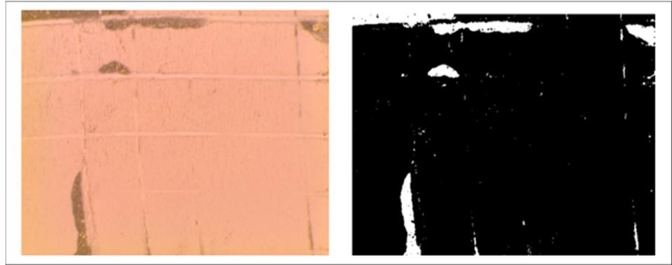
**Figure A1.** Image analysis example for the composite with polymer derived ceramics after crosscut test.
