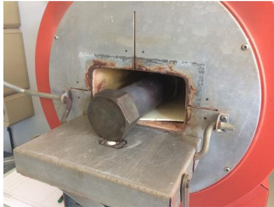
**Figure 2.** Small representative component coated with protective layer and filled with molten AlSi<sub>12</sub>.
