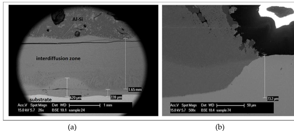
**Figure A4.** SEM micrograph. (a) Thickness of the intermetallic layers after 1200 h of aging with a TiAlN coating. (b) Diffusion of aluminum at some points—bad durability of the coating based on boron nitride.
