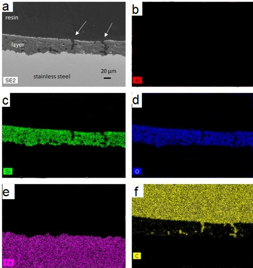
**Figure 10.** (a) SEM image of the protective layer on the 304 L tube after aging during 600 h at 700 °C in liquid AlSi<sub>12</sub> (300 X magnification) and EDS analysis of Al (b), Si (c), O (d), Fe (e), and C (f).
