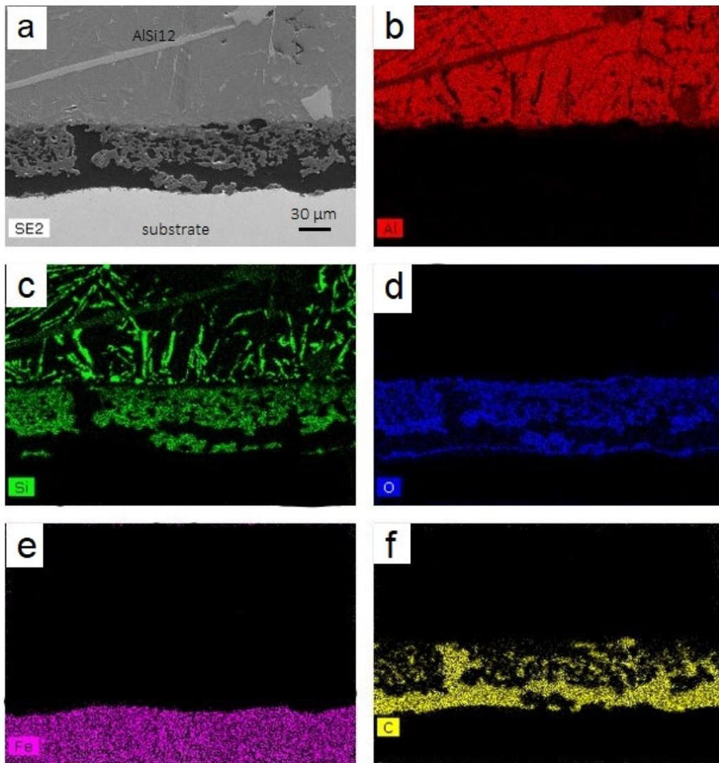
**Figure 7.** (a) Cross-sectional SEM observation of the protective layer coated on the 304L substrate after 600 h at 700 °C in AlSi<sub>12</sub> (300 X magnification) and EDS analysis of Al (b), Si (c), O (d), Fe (e), and C (f).
