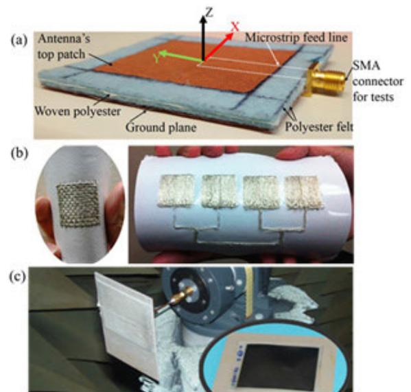
**FIGURE 4.** Textile-based patch antennas realized using: (a) adhesive backed conductive panel on conductive fabrics [79], (b) embroidery of conductive thread [95], (c) inkjet printing on interface layer [18].
