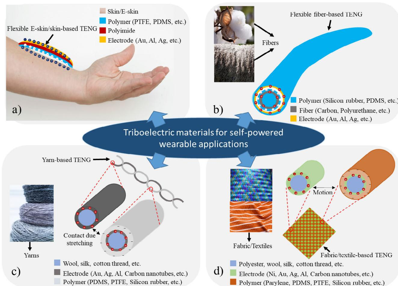
**FIGURE 7. TENG for self-powered wearable applications: (a) Skin-based TENG with triboelectric contact between polymer-skin. (b) Fiber-based TENG with triboelectric contact between conductor-polymer/fibre. (c) Yarn-based TENG with core-sheet yarn with triboelectric contact between yarn/conductor-polymer/conductor/yarn. (d) Fabric/textile-based TENG with triboelectric contact between textile/conductor-polymer/conductor/textile.**
