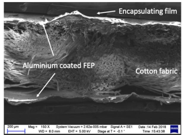
**FIGURE 5.** Cross-sectional scanning electron micrograph of a textile ferroelectret structure with the cotton layer sandwiched between the FEP films with aluminum electrodes and protective encapsulation [132].
