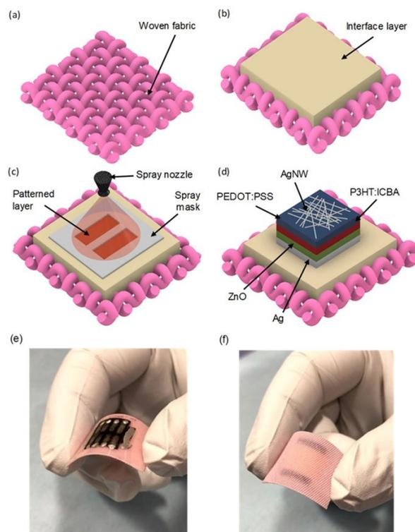
**FIGURE 8.** Isometric schematics illustrating the OSC structure and fabrication process. (a) Example woven fabric structure. (b) Screen printed interface layer on the fabric. (c) Spray coating process using a mask. (d) Final OSC on the interface coated fabric. (e) Photo of finished OSC. (f) Photo of underside of textile substrate [221].
