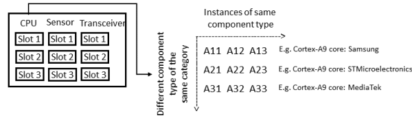
Fig. 3: Design-space definition for HW architecture
