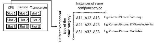
Fig. 3: Design-space definition for HW architecture
