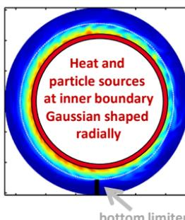
Mesh resolution on  $\frac{1}{2}$  torus:  $(\psi, \theta, \phi)$   $64 \times 512 \times 64$
