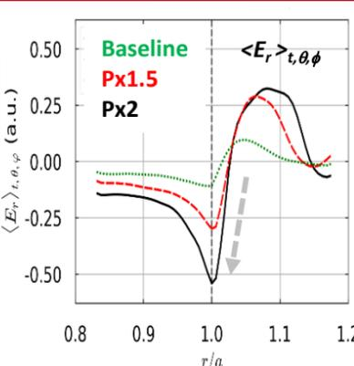
$E_r$  shear max in TOKAM3X simulations (w/o recycling) systematically @ few Larmor radii outside separatrix, in near SOL region similar to [Chanin PPCF 2017]
