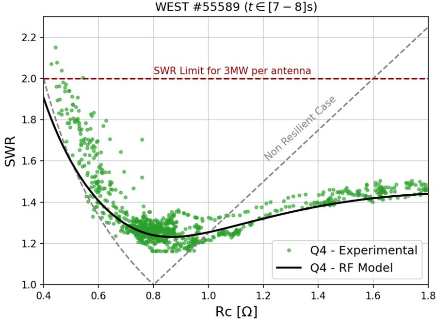
**Figure 9.** Standing Wave Ratio (SWR) versus coupling resistance ( $R_c$ ) for the WEST ICRH antenna Q4 (WEST pulse #55589) and RF modelling (plain line). The behaviour of a non-resilient antenna is indicated for reference (dashed line).
