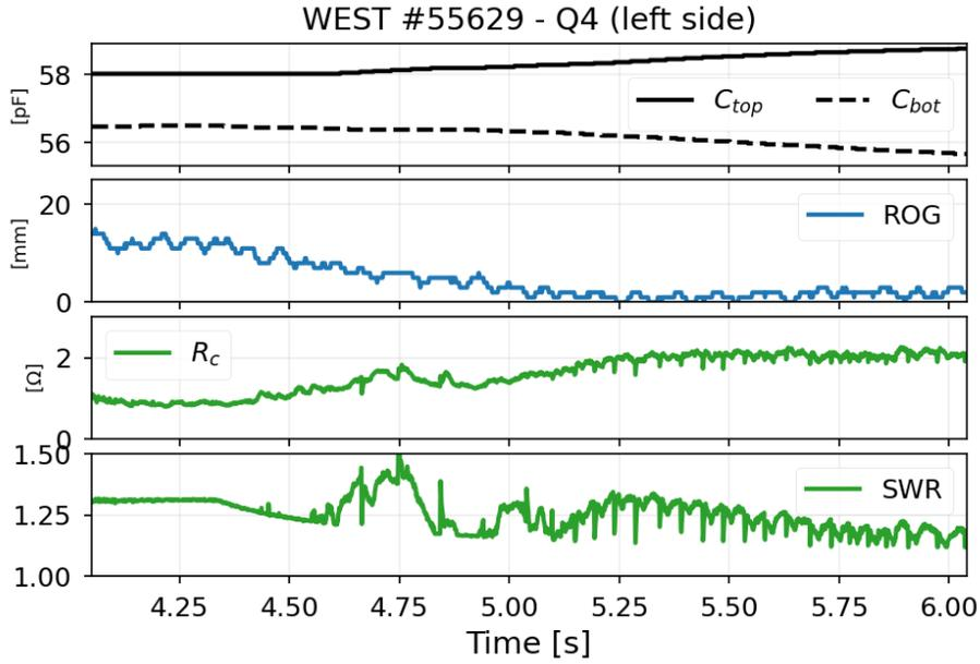
Figure 11. Example of real-time matching: As the Radial Outer Gap (ROG) of the plasma decreases, the coupling resistance ( $R_c$ ) increases and the capacitors move to improve the antenna matching (SWR decreases toward 1).
