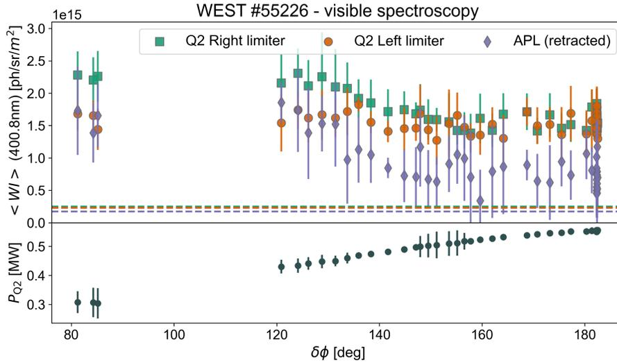
**Figure 15.** Averaged W-I brightness on the Q2 lateral limiters and the Antenna Protection Limiter (APL) during a toroidal phase scan of the Q2 antenna. Dashed lines correspond to the brightness level during the ohmic phase. The evolution of the average coupled power is also illustrated.
