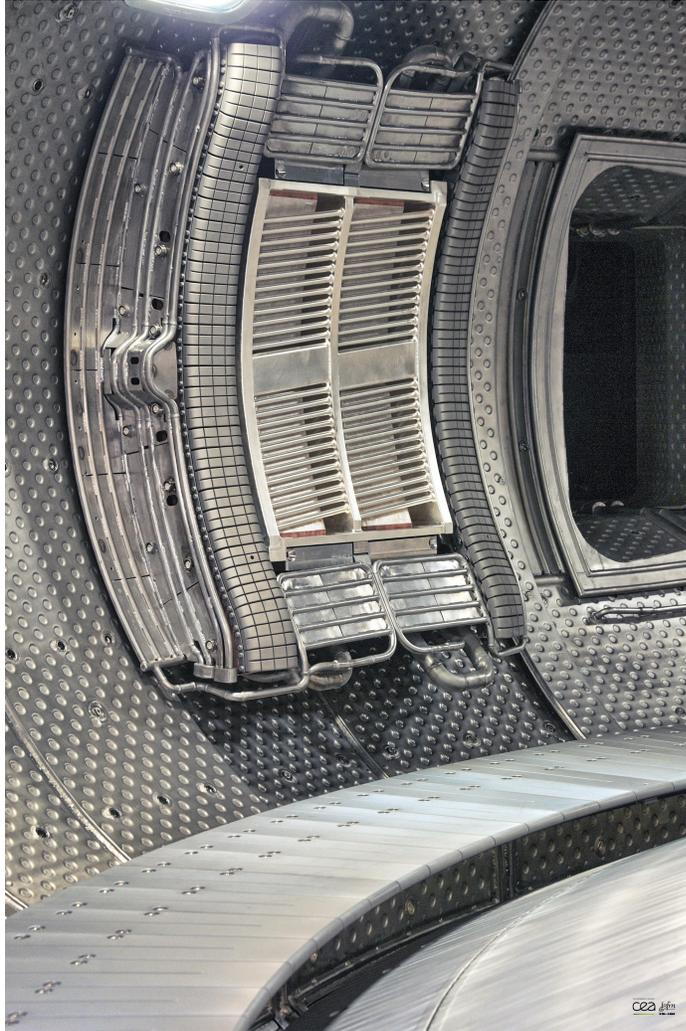
**Figure 4.** Picture of a WEST ICRH antenna inside the WEST machine, surrounded by its lateral W-coated limiters and steady-state heat flux shields
