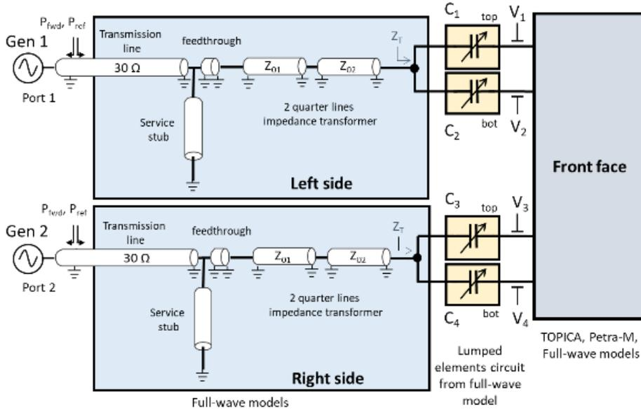
Figure 2. Block diagram of a WEST ICRH antenna.
