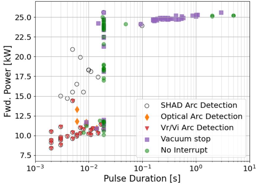
**Figure 7.** Example of vacuum conditioning process (from Q1 antenna in 2020), with mean strap voltage as a function of the RF pulse duration. RF conditioning starts at low forward power and duration (20 ms) and the power then the duration are increased until achieving stable pulses (no interruption).
