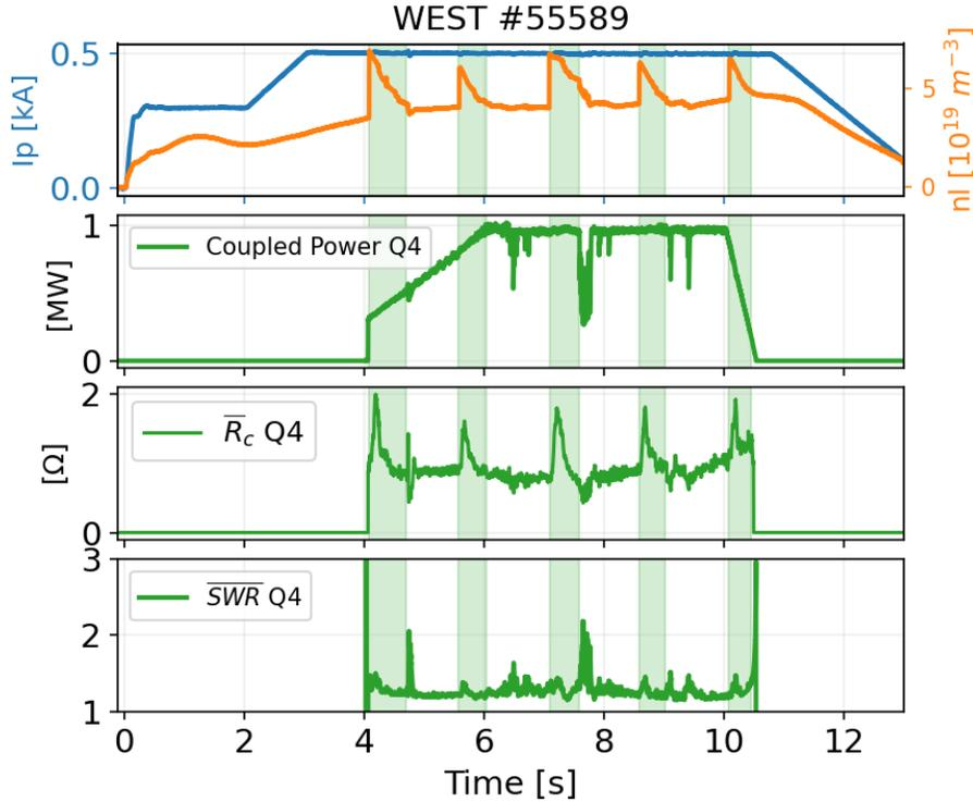
Figure 8. Antenna Load Resilience Demonstration using pellet injections.
