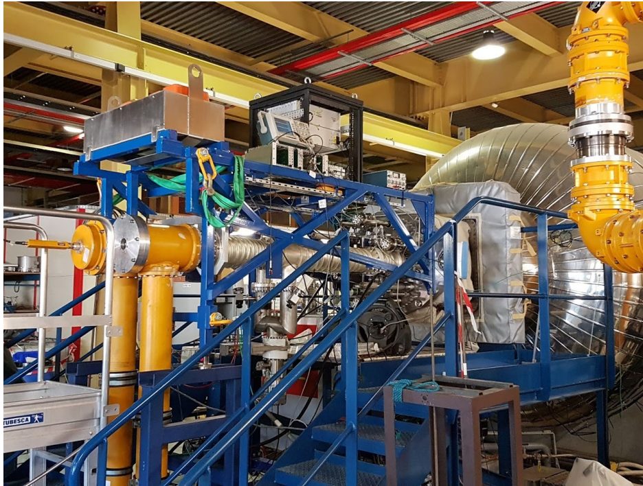
Figure 5. WEST ICRH Antenna Q4 installed in the TITAN vacuum chamber. The high power RF input (visible at the right side in yellow) is not yet connected to one antenna side.
