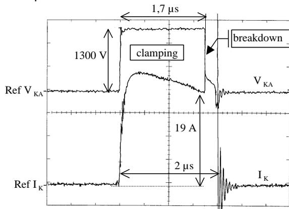
Figure 4 : Clamping and breakdown waveforms of a 1200 V diode
