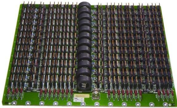
Figure 2 : 350 MOSFETs board switching 5 kV
