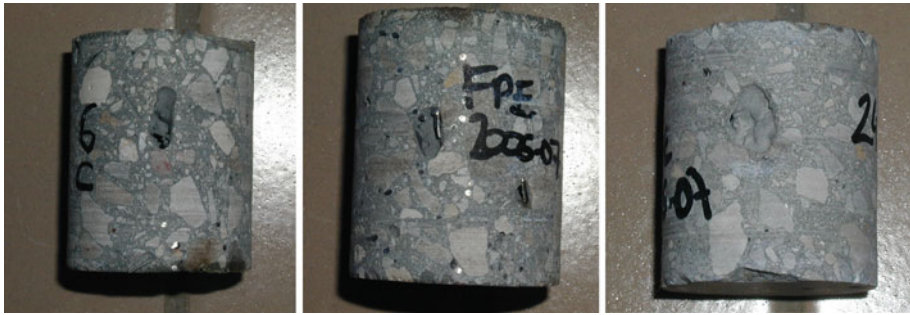
Fig. 9 Photographs of three different samples cored from the real waste package. Note the presence of entrapped air bubbles (samples diameter = 40 mm)
