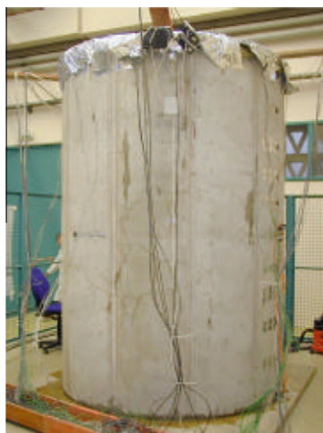
Fig. 1. General view of MAQBETH mock-up (left) and cylindrical steel reinforcement (right) [12].
