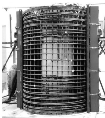
Fig. 1. General view of MAQBETH mock-up (left) and cylindrical steel reinforcement (right) [12].
