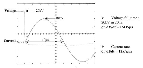
Nowadays, we are building a 100kV 10kA crowbar, consisting of 12 thyristors matrix in series. The final product would be finish and test during January 2000. It will not exceed 90cm high. This product will be presented in the final paper.
