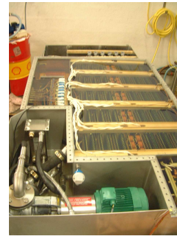
Fig. 5 30 kV 30 kA switch for excimer laser.
