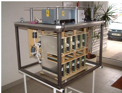
Fig. 7 High voltage serial protection switch for megawatt power supplies
