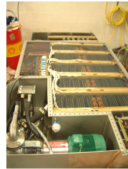
Fig. 5 30 kV 30 kA switch for excimer laser.
