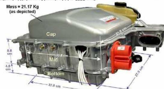
Volume (minus bus terminal/connector areas) = cap vol + mid vol + bottom vol
