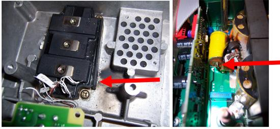
**Fig. 4.** IGBT and polypropylene capacitor having overheated
