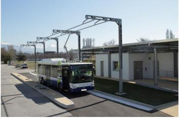
Figure 1: plug-in hybrid bus
