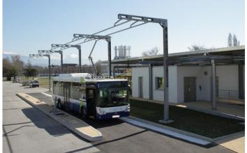
Figure 8: CEA 350kW charge station
