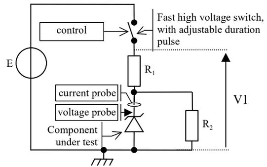
**Fig. 9:** Benchmark diagram for rectangular avalanche current shape
