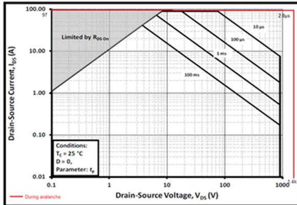
**Fig.16:** Device n°3 safe operating area during avalanche
