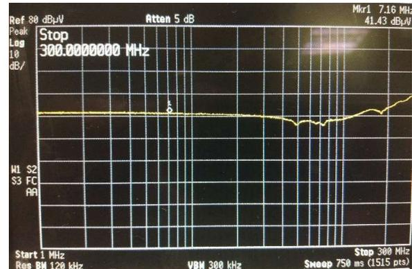
**Fig.13:** Bandwidth of the 5kΩ probe
