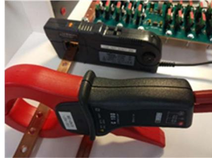
**Fig. 7:** Current measurement qualification
