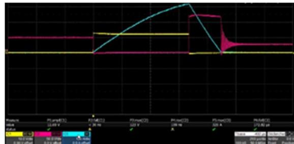
**Fig. 2:** Avalanche of three MOSFETs in parallel
