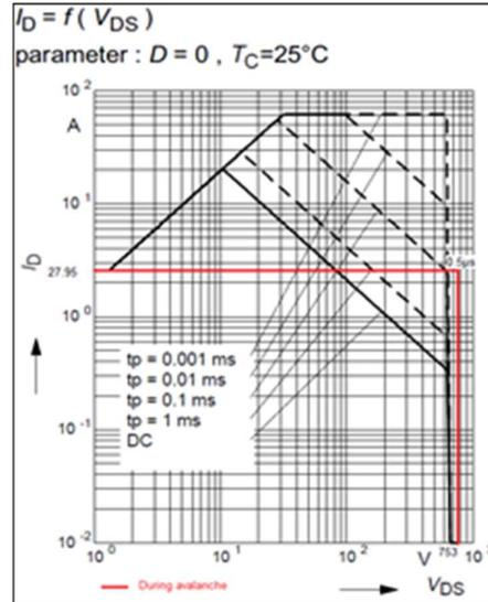
**Fig.15:** Device n°2 safe operating area during avalanche
