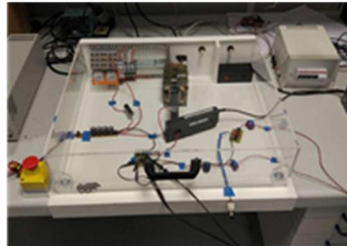
**Fig. 1:** Test of three MOSFETs in parallel
