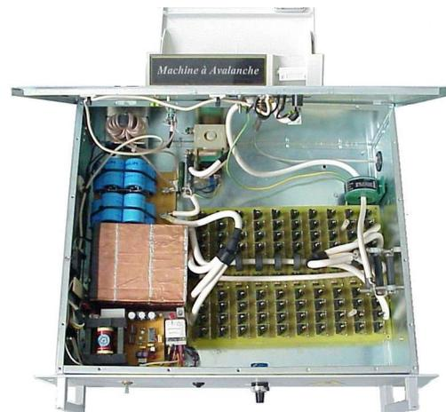
**Fig. 10:** Avalanche machine with the high voltage switch
