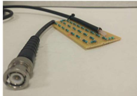
**Fig.12:** Handmade 5kΩ probe
