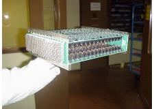
**Fig. 5:** 10 kV 500A Turn on, turn off and short circuit proof switch, diodes side On the figure 5, the horizontally PCBs are the MOSFET ones, the vertically one is the antiparallel high voltage diode.
