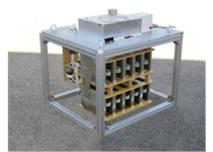
**Fig. 7:** 100 kV 25 A Turn on, turn off and short circuit proof switch for Tore Supra.
