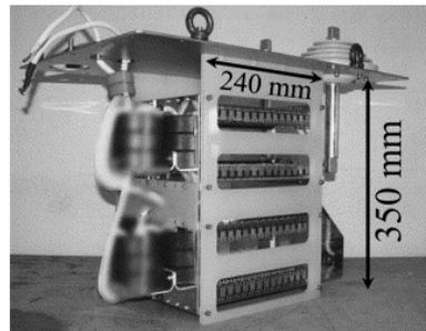
**Fig. 7:** 40 kV 10 kA Crowbar switch with thyristors Matrix
