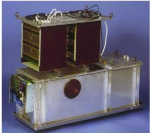
25 kV 1600 A switch for laser CENTRALP
