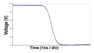
With this technology of driver it's possible to have MOSFETs in series, in parallel and in matrix. Now a 2 kV 1 ns fall time switch (in 50 ohms) is under development.
