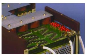
On the right part of the photograph is the high voltage probe with two high voltage resistors and small standard capacitors in series. It's a low cost solution for voltage measurement.
