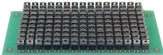
In the laser switch, a 3 A 60 kV diode is used between the transformer and the main capacitors. This diode is on the left part of the photograph.
