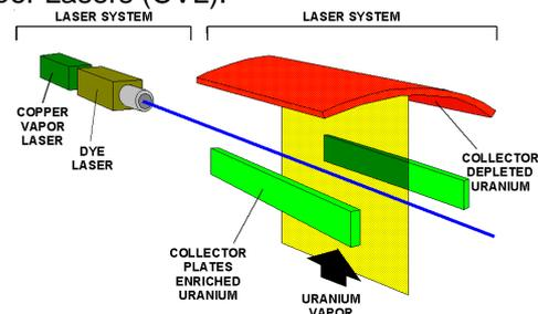
A SILVA enrichment module includes a laser system, whose photons, after an appropriate optical conditioning, irradiate a metallic vapor obtained by intense focalized heating generated by an electron beam.
