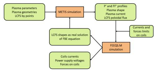
Figure 4 – Workflow combining METIS and FEEQS. In the case of the present simulations, METIS is run twice. In the first run, the LCFS is given by points; in the second run, the LCFS is computed and the full solution of the free-boundary equilibrium equation obtained by FEEQS is used.
