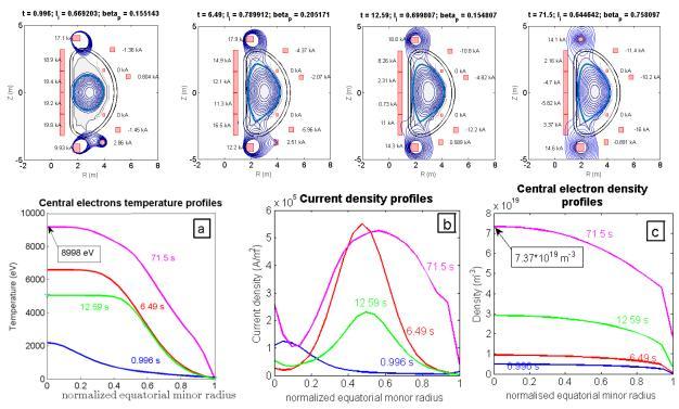
Figure 10 – Top: four plasma equilibria computed by FEEQS. From left to right the equilibrium corresponds to the time just before the x-point formation, the time after the x-point formation, the H-mode transition and a generic time during the flat-top. Bottom: The central electron temperature (a), current density (b) and density (c) profiles corresponding to the four equilibria shown in the top panels. x is the normalized Lao coordinate (normalized equatorial minor radius) [14].
