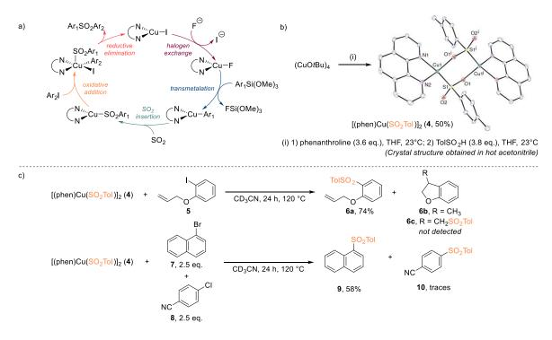
**Scheme 4.** (a) Proposed pathway for the mechanism of the reaction. (b) Synthesis of  $[(phen)Cu(SO_2-C_6H_4-CH_3)]_2$  (4). (c) Mechanistic control experiments: radical clock experiment with 2-(allyloxy)iodobenzene and substrate-competition study between 1-bromonaphthalene and 4-chlorobenzonitrile. Yields measured by <sup>1</sup>H NMR (internal standard: mesitylene).
