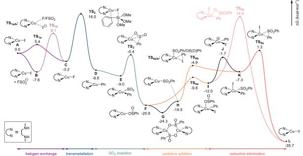
**Scheme 5.** DFT-calculated energy profile for the reaction. Level of theory: B3LYP-D3/6-311+G(d) (C, H, O, N, F), 6-311++G(d,p) (S, Si), SDD for Cu and def2-TZVP for I, PCM was used for CH<sub>3</sub>CN solvation. Given values correspond to Gibbs free energies (in kcal·mol<sup>-1</sup>). Since SO<sub>2</sub> decoordinates from DABCO without any transition state, free SO<sub>2</sub> was considered to compute transition states.
