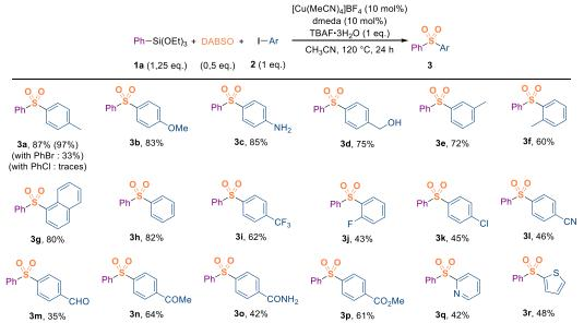
Scheme 2. Substrate scope in organohalides. Reaction conditions: phenyl(triethoxy)silane (1a, 1.25 mmol, 1.25 eq.), electrophile (1.0 mmol, 1.0 eq.), DABSO (0.50 mmol, 0.50 eq.), TBAF·3H<sub>2</sub>O (1.0 mmol, 1.0 eq.), Cu(MeCN)<sub>4</sub>BF<sub>4</sub> (0.10 mmol, 10 mol%), dmeda (0.10 mmol, 10 mol%), CH<sub>3</sub>CN (4 mL), 120 °C, 24 h. Isolated yields. Yields within parentheses were measured by <sup>1</sup>H NMR on 0.1 mmol scale (internal standard: mesitylene)
