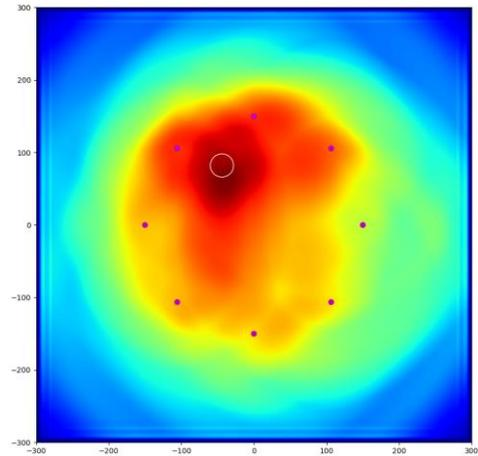
**FIGURE 2:** Passive imaging (vibration generated by compressed air, reception by FBGs) of a defect represented by the white circle in a CFRP plate using the Excitelet algorithm and 8 FBG sensors. Passive signals are deconvolved to reconstruct a 5-cycle tone burst at 30 kHz
