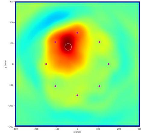
**FIGURE 1:** Active hybrid imaging (Emission by piezoelectric, reception by FBGs) of a defect represented by the white circle in a CFRP plate using the Excitelet algorithm and 8 piezoelectric sensors. The excitation is a 5-cycle tone burst at 30 kHz.
