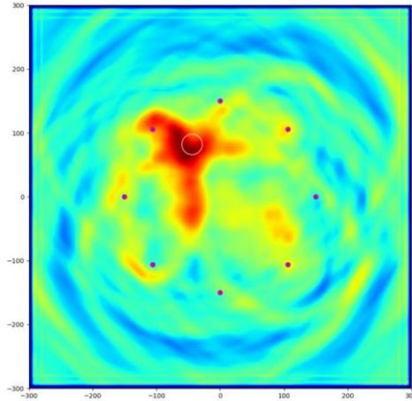
**FIGURE 3:** Passive imaging (vibration generated by compressed air, reception by FBGs) of a defect represented by the white circle in a CFRP plate using the Excitelet algorithm and 8 FBG sensors. Passive signals are deconvolved to reconstruct a 2-cycle tone burst at 30 kHz
