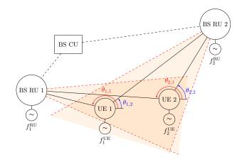
Figure 1. System model with two UEs.
