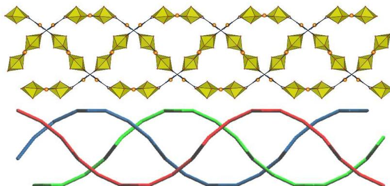
Depending on the structure-directing species present, uranyl cations associate with 2,5-thiophenedicarboxylate ligands to form mono- or diperiodic coordination polymers of varying geometry. In particular, honeycomb networks are found either associated with columns of counterions in polythreading-like fashion, or 3-fold interpenetrated, an entanglement mode not previously known in this family.
