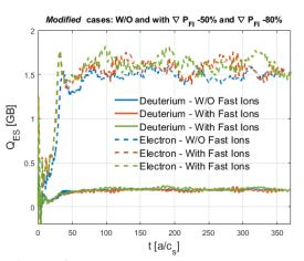
**Figure 2.** Time trace comparison between the electrostatic heat fluxes with and without fast ions of electron and thermal deuterium species for the 'modified' case [12].
