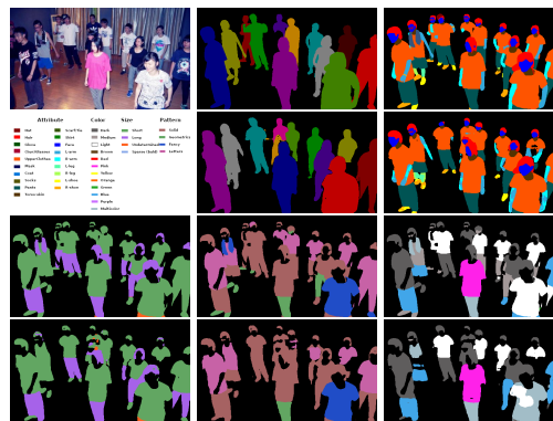
Fig. 1: Example of CCIHP ground truths (1st and 3rd rows) and our model predictions (2nd and 4th rows). First two rows: RGB image and legends, human instance, and semantic attribute maps. Last two rows: size, pattern and color maps.
