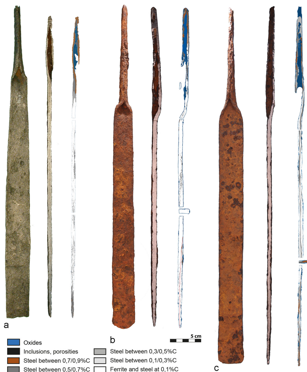
Figure 4 : Metallographi analyses. The sections analysed: a SAO 85.01.01B (Saint Marcel — Saône River), made by simple deformation of a single mass of metal. b SAL.24 (Saint Thiébaud — region of Salins-les-Bains), with onefold. c VAL.01 (Valempoulières — region of Salins-les-Bains), manufactured by successive folding
