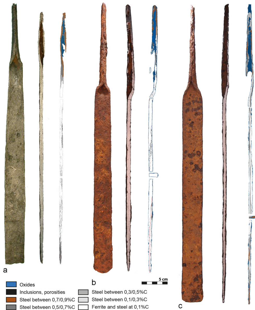
Figure 4 : Metallography analyses. The sections analysed: a SAO 85.01.01B (Saint Marcel — Saône River), made by simple deformation of a single mass of metal. b SAL.24 (Saint Thiébaud — region of Salins-les-Bains), with onefold. c VAL.01 (Valempoulières — region of Salins-les-Bains), manufactured by successive folding
