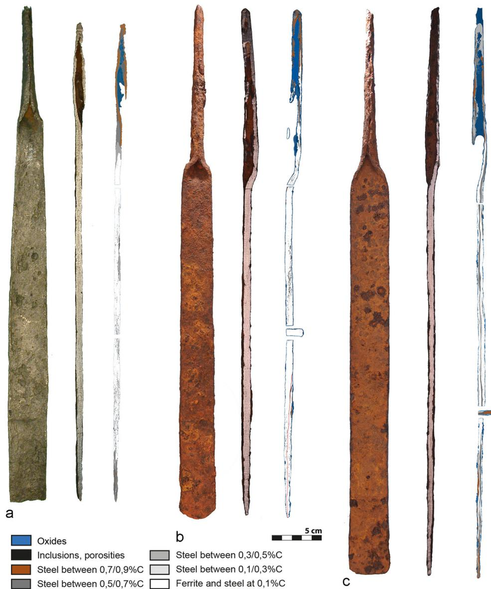
Figure 4 : Metallographi canalses. The sections analysed: a SAO 85.01.01B (Saint Marcel — Saône River), made by simple deformation of a single mass of metal. b SAL.24 (Saint Thiébaud — region of Salins-les-Bains), with onefold. c VAL.01 (Valempoulières — region of Salins-les-Bains), manufactured by successive folding
