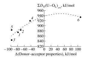
**Fig. 4.** Dependence of the donor-acceptor properties ( $\Delta$  value) of the substituting ligand on the total bond energy of bonds U–O<sub>I</sub> for complexes *1*–6.
