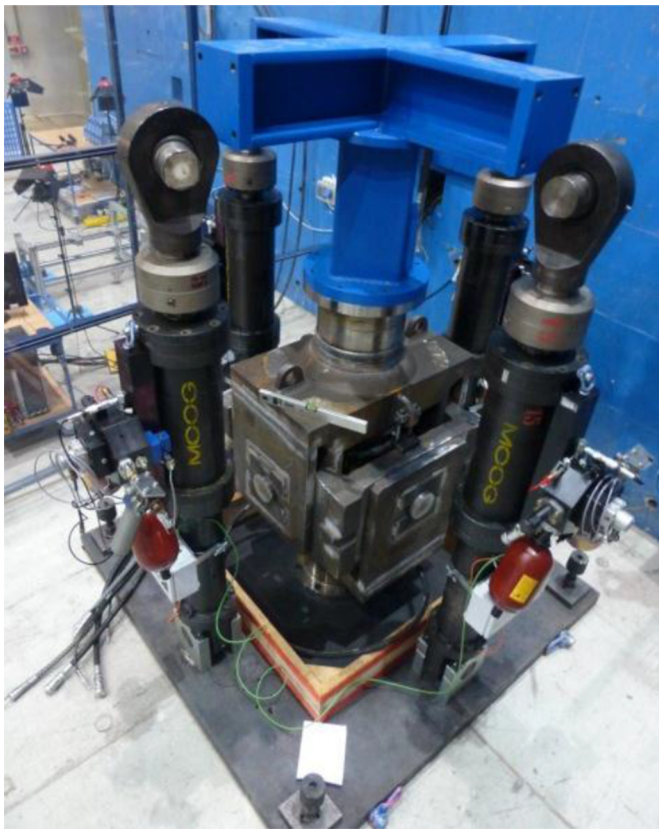
Fig. 5. Full scale pipeline expansion joint during seismic tests at the ELSA laboratory of the JRC of Ispra.
