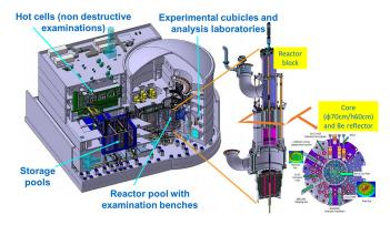
Fig. 2. General structure of the JHR.
