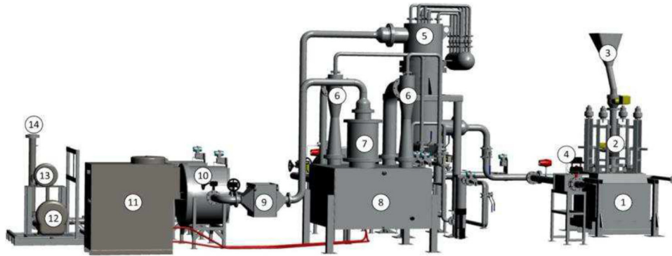
Fig. 6. The GeoMelt system installed at the NNL Central Laboratory. (1. ICV melter, 2. feed chute, 3. feed hopper, 4. connection to off-gas, 5. sintered metal filter, 6. scrubber column, 7. demister, 8. scrubber tank, 9. off-gas heater, 10. HEPA filtration, 11. cooler, 12. off-gas blower, 13. back-up blower and 14. vent discharge).
