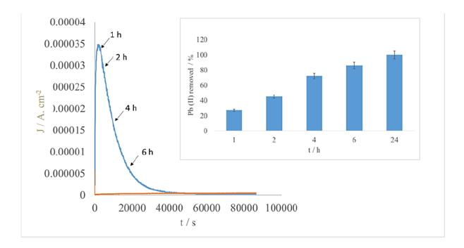
**Figure 4:** Current densities measured during electrochemical treatments for two solutions with  $[Pb(II)] = 27 \text{ mg. } L^{-1}$  (blue curve) and without the presence of Pb(II) (red curve): E imposed = 0.7V; pH  $\approx$  4.2 by adding NaOH (1M); with stirring, at room temperature, for 24 h, S (SnO<sub>2</sub>) = 3 cm<sup>2</sup>. *Insertion*: Percentages of Pb(II) removed as function of the treatment duration for solutions containing initially 27 mg. L<sup>-1</sup>.
