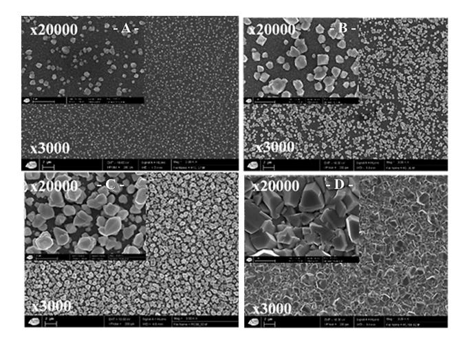
**Figure 7:** SEM observations of adherent thin films obtained after electrochemical treatment of solutions with different initial Pb(II) concentrations (E imposed = 0.7 V, pH  $\approx$  4.2 by adding NaOH (1M), with stirring; S (SnO<sub>2</sub>) = 3 cm<sup>2</sup>; at room temperature) during 24 h for (**A**) 1 mg.L<sup>-1</sup>; (**B**) 5 mg.L<sup>-1</sup> and (**C**) 27 mg.L<sup>-1</sup>, and 48 h for (**D**) 100 mg.L<sup>-1</sup>. Scale (x 3000: 0.3 cm = 2 µm) and (x 2000: 0.6 cm = 1 µm)
