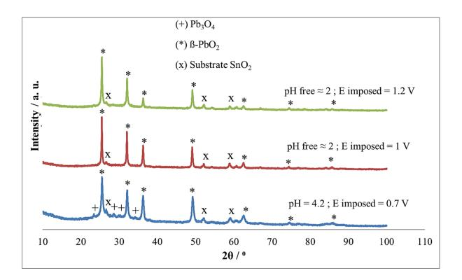
**Figure 2**: X-ray diffractograms of the adherent thin films obtained after the electrochemical treatment of a lead solution ( $[Pb(II)] = 27 \text{ mg.L}^{-1}$ ), for different values of imposed potentials and pH (pH free  $\approx 2$  and pH adjusted to 4.2 by adding of NaOH (1M)), at room temperature, with stirring of the solution (250 rpm) for 24 hours. S (SnO<sub>2</sub>) = 3 cm<sup>2</sup>
