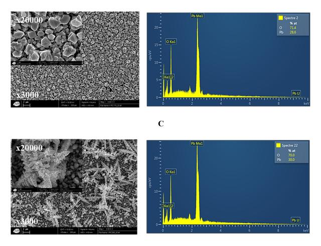
**Figure 3:** SEM observations and analyzes by EDS of the adherent thin films obtained after the electrochemical treatment of a lead solution ([Pb(II)] = 27 mg. L<sup>-1</sup>), at room temperature, with stirring, for 24 hours, with different values of imposed potential and pH, S (SnO<sub>2</sub>) = 3 cm<sup>2</sup>. (A) pH = 4.2, E = 0.7 V; (B) free pH  $\approx$  2, E = 1 V; (C) free pH  $\approx$  2, E = 1.2 V. Scale (x3000: 0.3 cm = 2 µm) and (x 20000: 0.6 cm = 1 µm).
