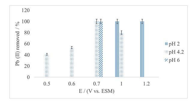
**Figure 1:** Percentages of Pb(II) removed according to the imposed potential for a solution of  $[Pb(II)] = 27 \text{ mg.L}^{-1}$ , at room temperature, with stirring of the solution (250 rpm) for 24 hours. S (SnO<sub>2</sub>) = 3 cm<sup>2</sup>
