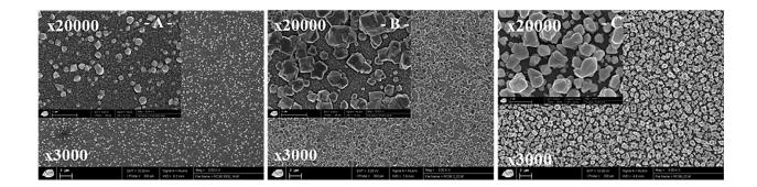
**Figure 5:** Observations by SEM of adherent thin films obtained after the electrochemical treatment at E imposed = 0.7V;  $[Pb(II)] = 27 \text{ mg. } \text{L}^{-1}$ ; pH = 4.2 by adding NaOH (1M); with stirring at 250 rpm, at room temperature, S (SnO<sub>2</sub>) = 3 cm<sup>2</sup>, after (A) 1 h; (B) 2 h, and (C) 24 h. Scale (x 3000: 0.3 cm = 2  $\mu$ m) and (x 2000: 0.6 cm = 1  $\mu$ m)
