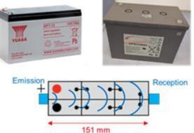
Figure 2: top – pictures of the two different types of AGM –type lead acid batteries studied. Bottom: drawing that shows the location of the transducers (Emission – Reception); example on the Yuasa NP7-12 battery.
