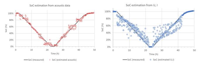
Figure 4 : Estimation of the state of charge of a GNB Sprinter XP6V2800 battery during cycling at ~C/20, using a simple machine learning algorithm. Left : estimation from acoustic datas. Right : estimation from the battery voltage and the current passing through the battery.
