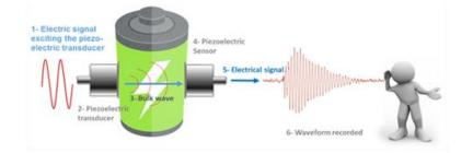
Figure 1 : working principle of the acoustic interrogation characterization technique
