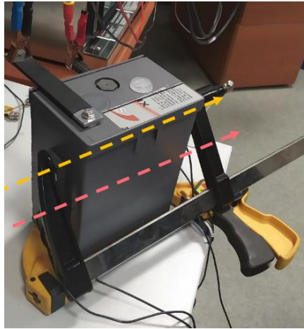
Measurements conducted on a cell of the battery (2 V / 195 Ah)
