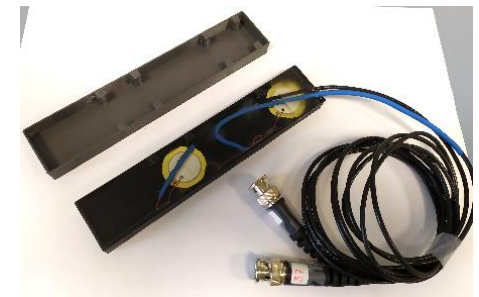
Coaxial wiring and BNC connections Transducers imbedded in a 3D printed holder using epoxy resin for sealing and mechanical fixation
