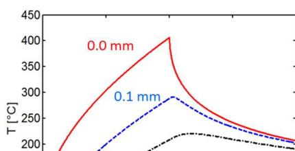
Figure 10. Thermal response of a 0.8 mm exposed leading edge to a square heat pulse of  $190 \text{ MW/m}^2$  applied for 1 ms (heat flux factor =  $6 \text{ MW m}^{-2} \text{ s}^{1/2}$ ). The temperature at the surface (0.0 mm, full curve) and at two depths below the surface (0.1 mm, dashed curve; 0.2 mm, dot-dash curve) are shown. The initial temperature is  $70^\circ\text{C}$ .
