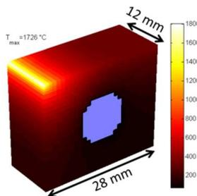
Figure 13. Surface temperature of a misaligned MB exposed for 5 s to a heat flux to the top surface  $q_{pk}=2.5 \text{ MW}/\text{m}^2$ . The 0.8 mm exposed leading edge is irradiated by the parallel heat flux which, when ion orbit effects are accounted for, peaks at  $q_{surf}=70 \text{ MW}/\text{m}^2$ . The 3D heat flux profile from which a toroidal slice was shown in Figure 12 was used for the surface boundary condition of this thermal calculation.
