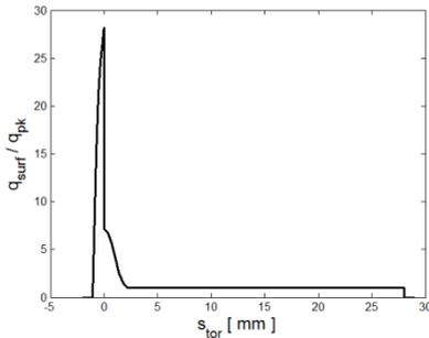
Figure 12. Toroidal profile of the heat flux to a misaligned WEST MB normalized by the heat flux to the top surface  $q_{pk}=2.5 \text{ MW}/\text{m}^2$ . The leading edge is at  $s_{tor}=0 \text{ mm}$ ; negative values correspond to the front face inside the toroidal gap. The MB is misaligned by  $+0.8 \text{ mm}$ .
