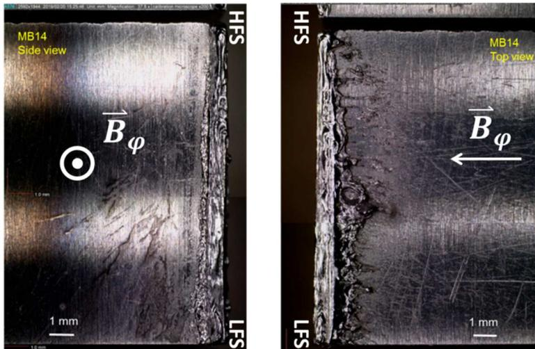
Figure 4. Side (left panel) and top (right panel) views of the trailing edge of MB#14. The images were taken after dismantling PFU#12 following the C3 experimental campaign. Melting of the leading edge to a depth about 1 mm and splashing of the melt layer over a few mm on the top surface are observed.
