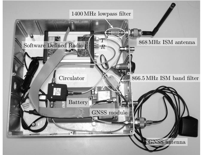
Fig. 2. Transceiver testbed composed of a SDR, radio frequency components, a GNSS module and a power supply.
