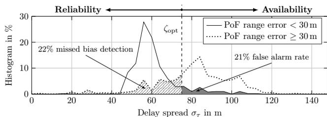
Fig. 7. Delay spread histograms for biased PoF ranging estimates detection.
