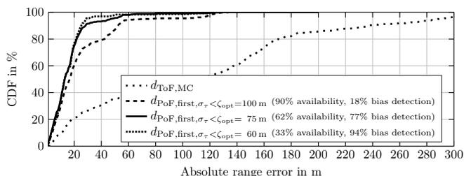
Fig. 8. Ranging errors for ToF and PoF estimation.
