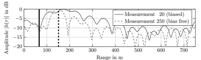
Fig. 6. Comparison of estimated channel impulse responses  $h(\tau)$  for a biased and bias free measurement. Vertical lines indicate true range.
