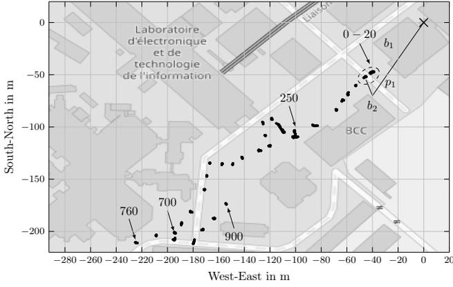
Fig. 4. GNSS ground truth positions ( $\cdot$ ) w.r.t. the roof testbed ( $\times$ ) at  $(0, 0)$ .
