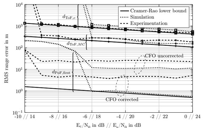
Fig. 3. Simulated and measured ranging error in a frequency flat channel with a signal bandwidth  $BW_{\text{sym}} = 10 \text{ kHz}$ ,  $C = 16$  channels, a virtual multi-channel bandwidth  $BW_{\text{virt}} = 3.0 \text{ MHz}$  and CFO.
