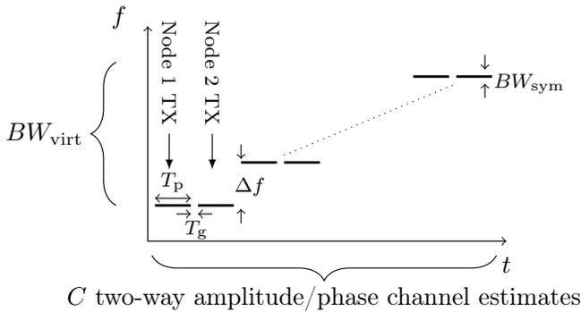
Fig. 1. Multi-channel ranging signaling process for  $C$  sequentially aggregated narrowband ( $BW_{\text{sym}}$ ) channels form a virtual bandwidth  $BW_{\text{virt}} = (C-1)\Delta f$ .
