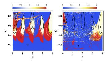
FIG. 1. Phase diagram in the presence of orbital effects. We plot the MP as a function of  $\tilde{\mu}$  and  $\tilde{V}_z$ . The black lines indicate the boundary of the phase diagram when the orbital effects are ignored. The g-factor  $g^*$  is taken to be 50 for the left panel and 10 for the right panel respectively. We consider  $\tilde{\Delta} = 0.4$ ,  $\tilde{\alpha} = 0.2$ .
