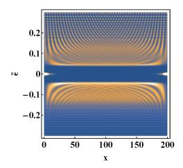
FIG. 9. The density of states plotted as a function of position x and dimensionless energy  $\tilde{\epsilon}$ . The bright spots at zero energy represent the "traditional pair" of MBS localized at the ends of the system in the absence of orbital effects. We set  $\tilde{\Delta} = 0.4$ ,  $\tilde{V}_Z = 0.5$ ,  $\tilde{\alpha} = 0.2$ .
