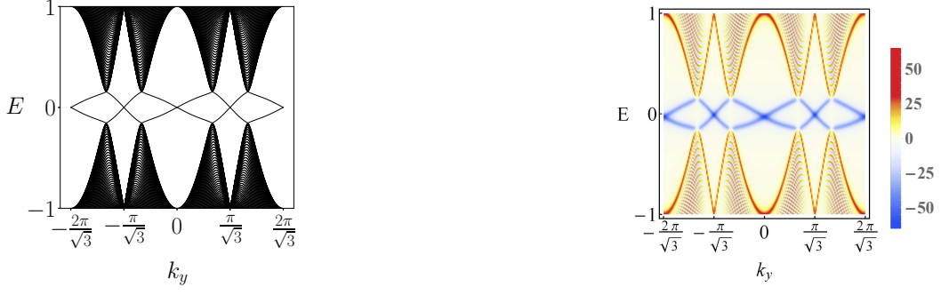
Figure 11. Left panel: energy spectrum obtained by an exact diagonalization of the Hamiltonian in Eq. (16) defined on a strip with one zigzag edge and one bearded edge. Right panel: the correction to the averaged spectral function due to the line impurity localized on either of the two sublattices. We consider U = 100 . For both plots, hopping amplitudes are taken to be t = 1, t_2 = 0.03
