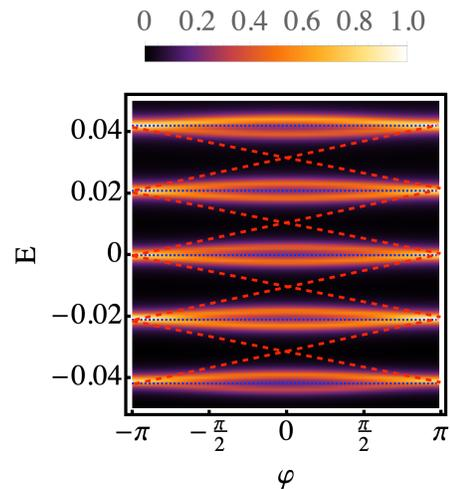
Figure 7. LDOS averaged over 6 sites  $x \in [90, 95]$ , plotted as a function of the phase difference  $\varphi$  on the horizontal axis and energy on the vertical axis. We set  $L = 200$ ,  $V_A = 3.5$  and  $\mu = 1.5$ . The perfect Andreev limit is denoted by the red dashed lines while the particle-in-the-box by the blue dotted lines.
