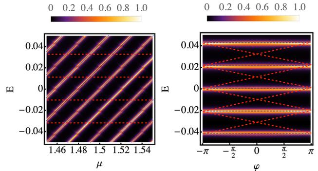
Figure 8. LDOS averaged over 6 sites  $x \in [90, 95]$ , plotted as a function of energy (vertical axis) and on the horizontal axis the chemical potential (left panel) and the SC phase difference (right panel). Here we set  $L = 200$ ,  $V_A = 10$ . In the left panel we fix  $\varphi = 0$ , whereas in the right panel  $\mu = 1.5$ . The perfect Andreev limit is denoted by the dashed red lines while the particle-in-the-box by the dotted blue lines.
