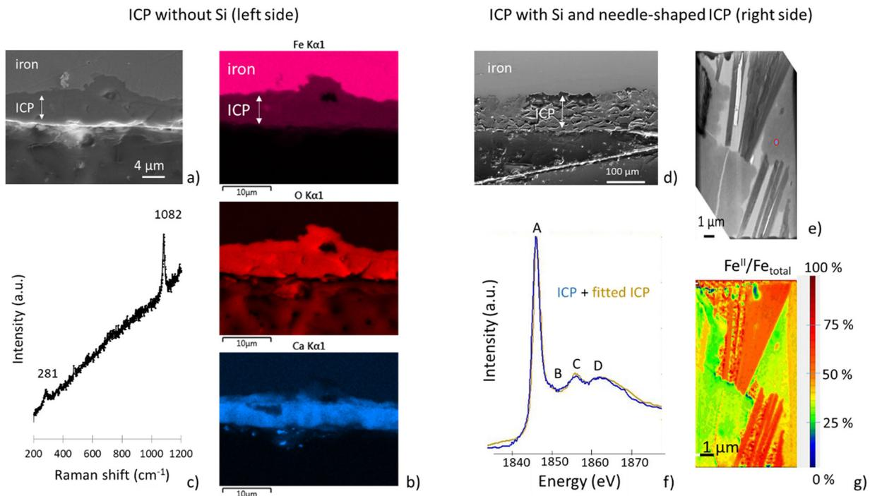
**Fig. 7** ICP characterizations. **a** SEM micrograph, **b** SEM-EDS elemental mapping and **c**  $\mu$ Raman analyses of ICP on the left side, without Si. **d** SEM micrograph and **e** TEM micrograph of ICP on the right side, i.e., containing Si or needle-shaped ICP. **f** STXM spectra at Si K-edge on ICP with silicon (blue) and fitted spectrum (brown). **g** quantitative Fe redox nanomapping obtained with STXM at Fe L-edge from micrograph in **e**.
