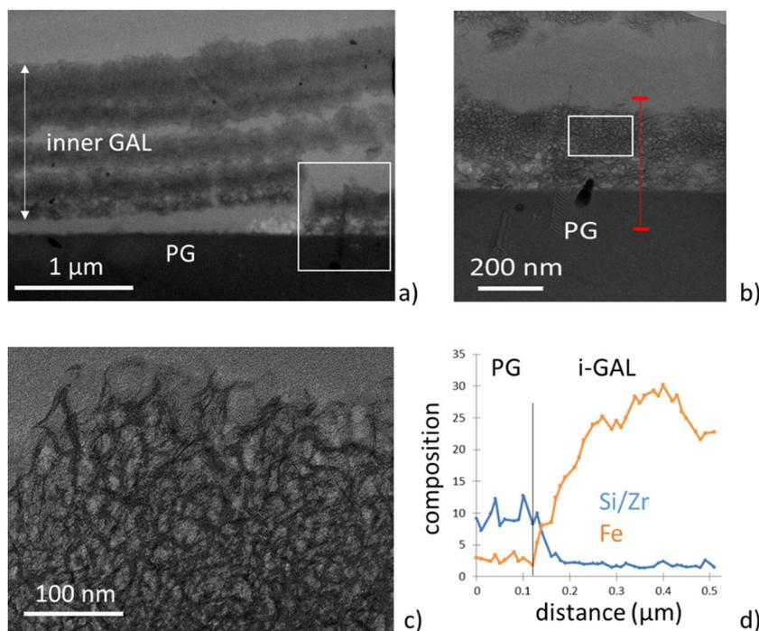
**Fig. 3** TEM analyses performed in the inner GAL. **a** TEM micrographs of the i-GAL evidencing several strata and location of the profile composition (red line) in the first stratum (**b**). In **c**, HRTEM in the first stratum of the i-GAL showing foliated aggregates compatible with the smectite morphology. In **d**, TEM-EDS profile composition (wt.%) obtained in the first stratum of the i-GAL highlighting the PG/i-GAL interface.
