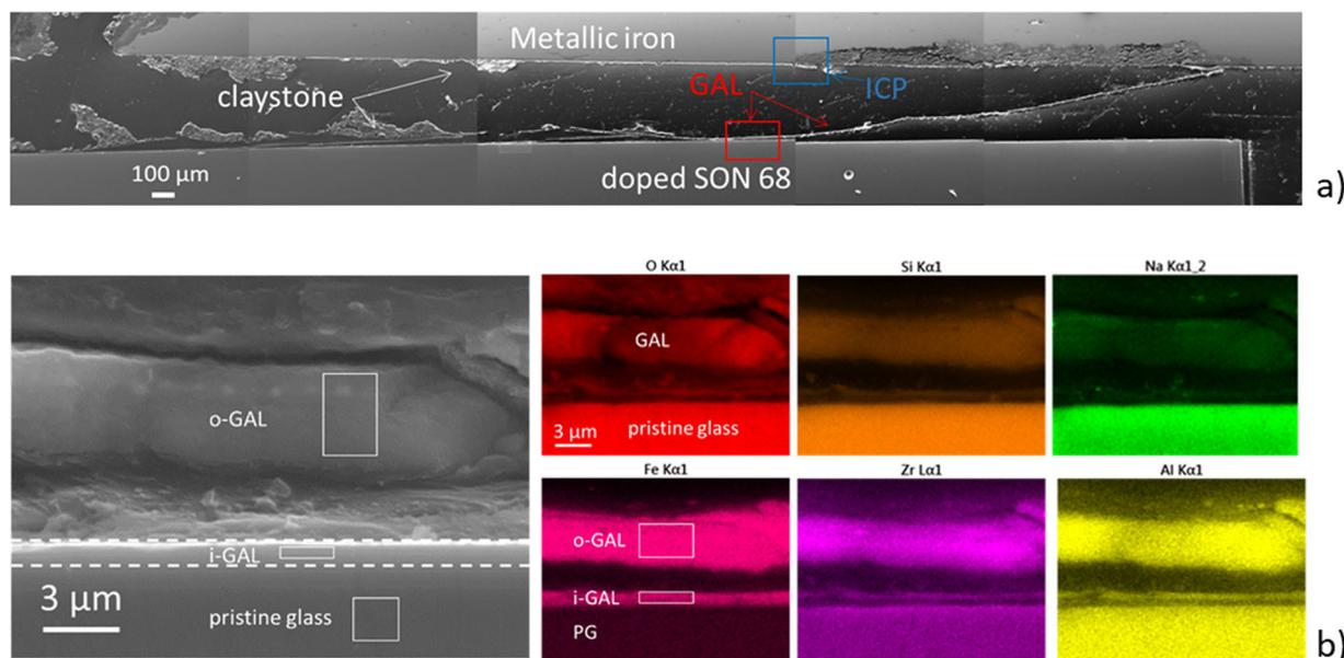
**Fig. 2** SEM analyses at the glass/iron interface. **a** SEM micrograph of the doped nuclear glass/iron interface. The rectangles indicate the areas studied in detail (i.e., GAL and ICP). **b** SEM micrograph and EDS elemental mapping of the doped glass surface. White squares indicate areas of EDS analyses (Table 1).
