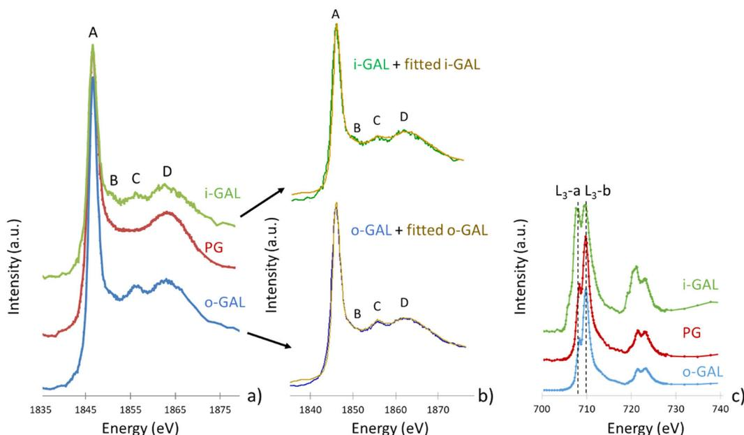
**Fig. 5** STXM analyses at Si K and Fe-L edges of the glass alteration layer. **a** Si K-edge spectra obtained in pristine glass, i-GAL and o-GAL and superposition of i-GAL and o-GAL spectra with corresponding fitted spectra (**b**). Fe L-edge spectra obtained in pristine glass, i-GAL and o-GAL (**c**).
