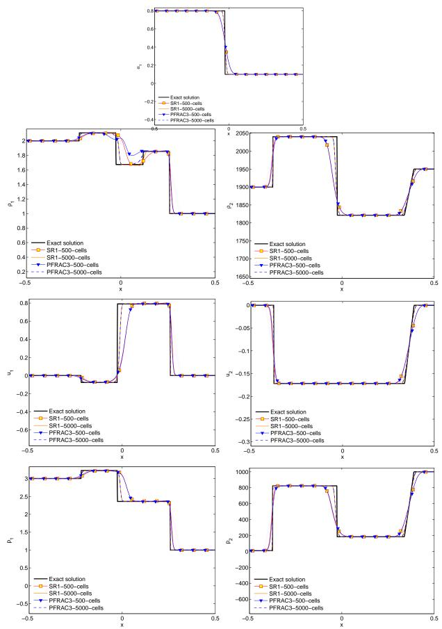
Figure 4. Approximate solutions for variables  $\alpha_v, \rho_k, u_k, p_k, k = l, v$  for test case 2 by Tokareva and Toro , using SR1, and PFRAC32 schemes with 500 and 5000 cells.  $CFL = 1/2, \ t = 0.15$
