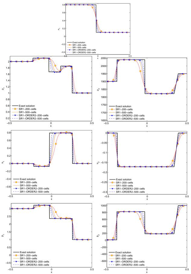
Figure 6. Approximate solutions for variables  $\alpha_v, \rho_k, u_k, p_k, k = l, v$  for test case 2 by Tokareva and Toro, for first and second-order schemes SR1, SR1-ORDER2, with 200, 500 cells, setting CFL = 1/2, t = 0.15
