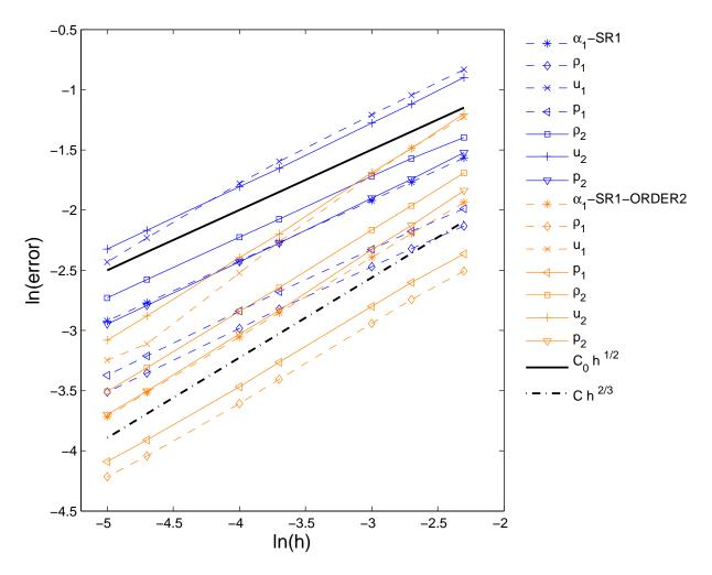
Figure 1. Convergence curves for  $\alpha_1, \rho_k, u_k, p_k, k=1,2$  for test case 1 by Schwendeman-Wahle-Kapila. Results have been obtained with first-order and second-order SR1 and SR1-ORDER2 schemes , setting: CFL=1/2, t=0.2. The black line is a reference  $C_oh^{1/2}$ .
