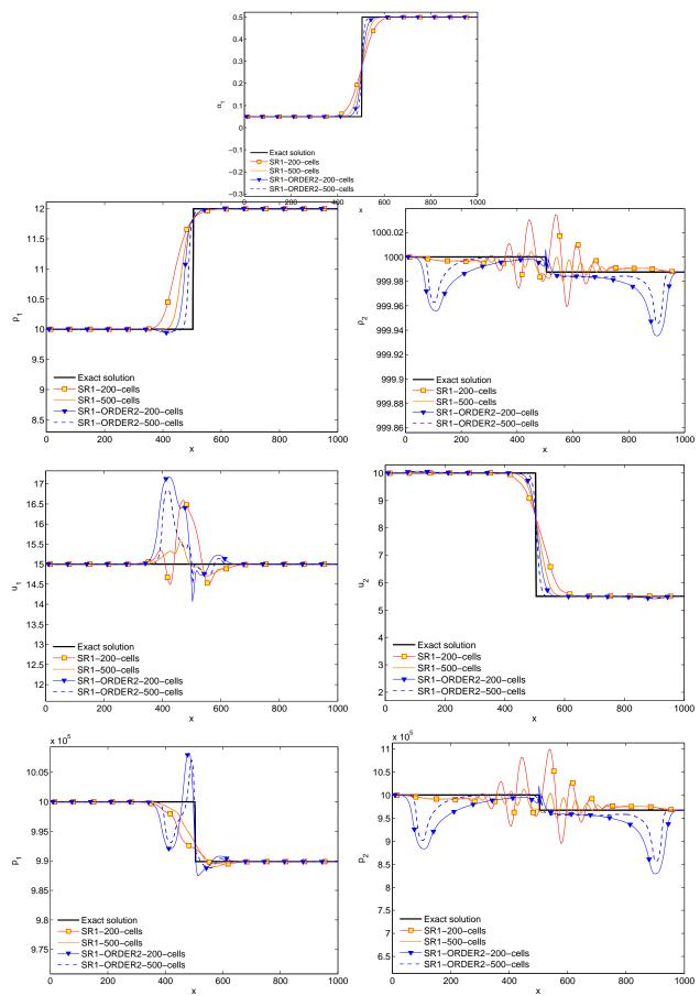
Figure 10. Approximate solutions for variables  $\alpha_v$ ,  $\rho_k$ ,  $u_k$ ,  $p_k$ , k=l, v for test case 3 of a moving VFW, using first and second-order schemes SR1, SR1-ORDER2 with meshes containing 200 and 500 cells ( CFL = 1/2, t = 0.25)
