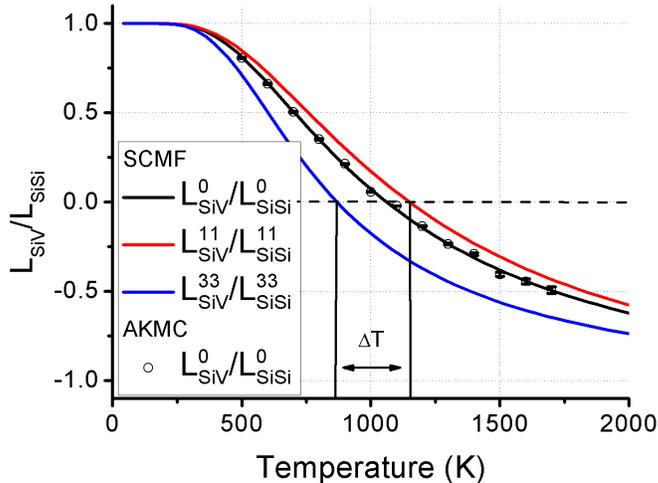
FIG. 8. (color online)  $L_{BV}/L_{BB}$  ratio for the Ni(Si) alloy in the absence of strain (solid line for SCMF results, circles for AKMC results) and under a tetragonal tensile strain  $\varepsilon_{33} = -2\varepsilon_{11} = -2\varepsilon_{22} = \varepsilon = 0.01$  as a function of the temperature in the  $[100]$  direction (dashed line) and in the  $[010]$  direction (dotted line). The error bars represent the statistical variance of AKMC simulations.
