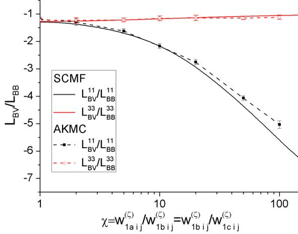
FIG. 5. Drag ratio  $L_{BV}/L_{BB}$  in the [001] direction and in the (001) plane of a model alloy under an elementary strain  $\varepsilon_{12}$  as a function of  $\chi$  (for all  $\zeta, i, j$ ,  $w_{1a ij}^{(\zeta)} = \chi$ ,  $w_{1b ij}^{(\zeta)} = 1$  and  $w_{1c ij}^{(\zeta)} = \chi^{-1}$ ). Symbols indicate results of AKMC simulations, with error bars computed from their statistical standard deviation, and the solid line is the SCMF result.
