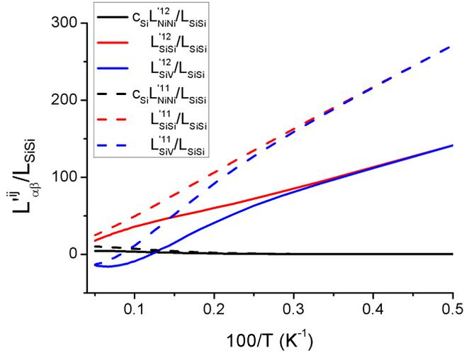
FIG. 9. (color online) Derivatives of the Onsager matrix of the Ni(Si) alloy with respect to strain. The  $L^{11}$  are dashed lines and the  $L^{12}$  terms are solid, with black for the matrix term, red for the impurity term and blue for the vacancy-impurity correlation.
