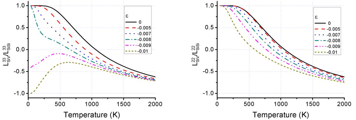
FIG. 10. (color online)  $L_{BV}/L_{BB}$  ratio for the Ni(Si) alloy under a tetragonal compressive strain  $\varepsilon_{33} = -2\varepsilon_{11} = -2\varepsilon_{22} = \varepsilon < 0$  as a function of the temperature and  $\varepsilon$  along the  $[100]$  direction (left) and the  $[010]$  directions (right).
