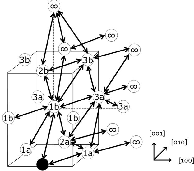
FIG. 6. Vacancy jump frequencies in a dilute FCC binary alloy with first, second and third NN interactions under a  $\varepsilon_{33}$  strain. Arrows indicate the direction of the vacancy jumps. The solute atom is represented by a filled circle, and on the other sites of the lattice the numbers describe the distance from the solute atom site with an  $\infty$  sign for the sites beyond the range of the interactions.
