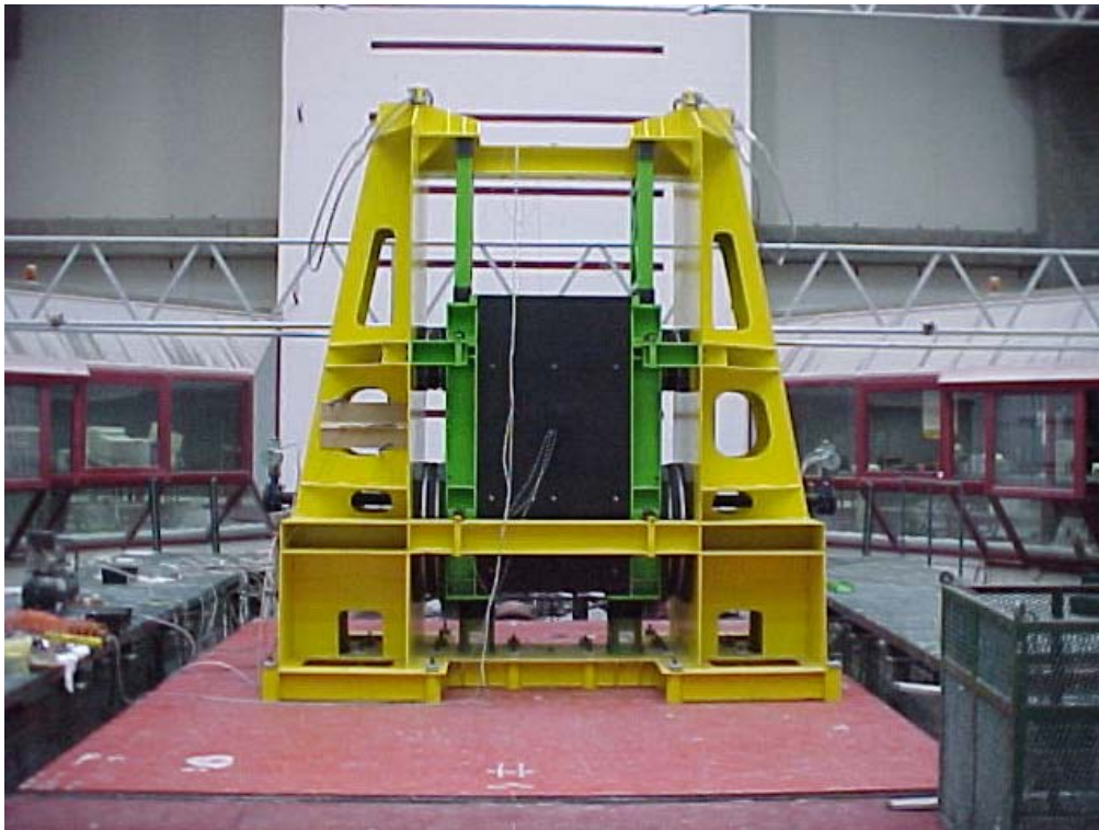
Photography 2 – View of the mock-up on the LNEC shaking table
