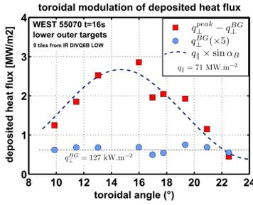
Figure 3: Toroidal profiles of the peak (red squares) and background components (blue circles) of the deposited heat flux along 9 tiles sitting on the lower outer divertor (see Fig.1). The dashed curve represents the geometrical projection of a uniform parallel heat flux, with  $\alpha_B$  the incidence angle of the local magnetic field on the divertor surface.
