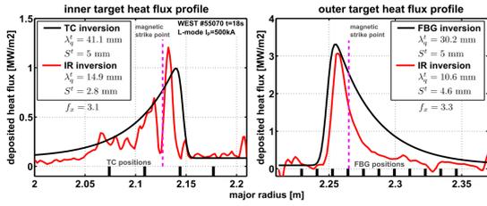
Figure 4: Radial profiles of the deposited heat fluxes from embedded measurements and IR inversion along the inner and outer targets (at the maximum ripple modulation). Black curves show the TC (inner) and FBG (outer) inversions with the prescribed analytical shape and red curves are for the IR inversion. Absolute positions of the embedded sensors are shown as black ticks at the bottom of profiles.
