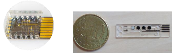
Fig. 7. Nanowire (left) and potentiometric (right) sensors brought to the project by partners
